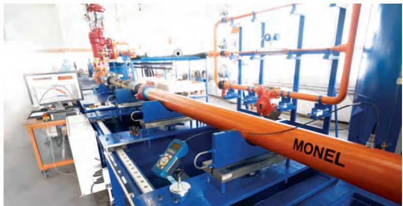
ESP hydraulics being tested at the Oil Dynamics GmbH factory in Germany
